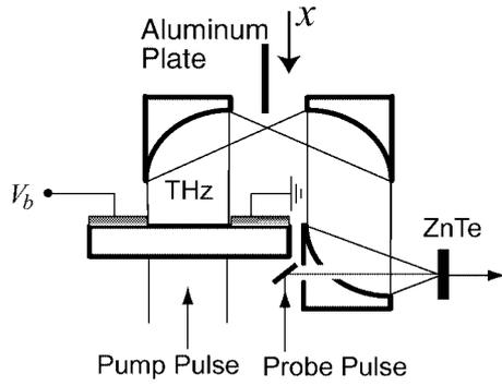
Fig. 2: The experimental setup for the knife edge measurement. Axis  $x$  is the path which the edge of the aluminum plate passes through. The origin of  $x$  is taken as the optical focus of the mirror.
