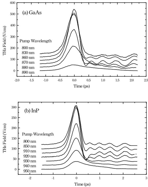
Fig. 2. Pump wavelength dependence of the THz waveforms obtained from (a) GaAs and (b) InP. The bias field applied to the materials was 6.7 kV/cm. The oscillations at positive times are due to absorption by water vapor in the air, and do not reflect electron dynamics.
