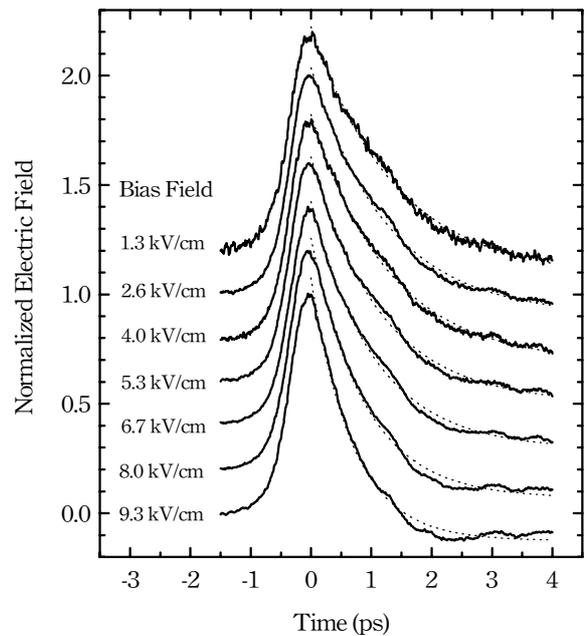
Fig. 3. Bias field dependence of the THz waveforms obtained from GaAs with 890-nm pumping.
