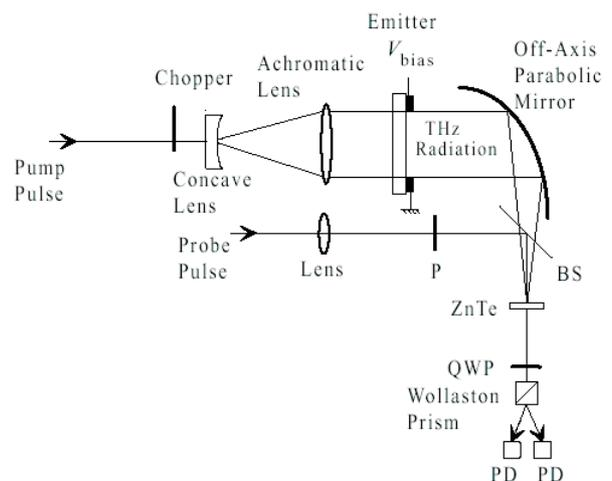
Fig. 1. Schematic of the experimental setup for the measurement of the THz radiation waveforms. P: polarizer, BS: beamsplitter, QWP: quarter-wave plate, and PD: photodiode.
