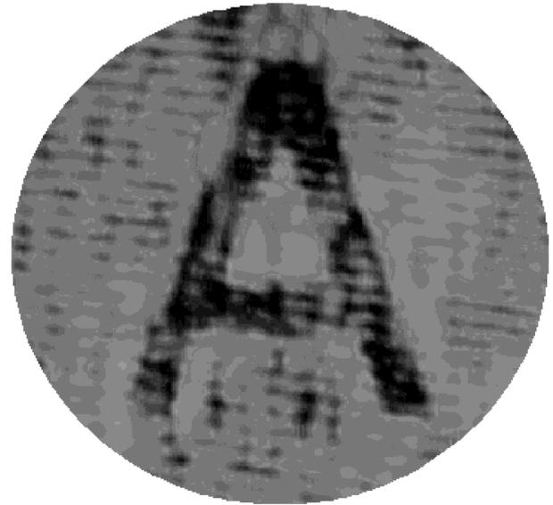
Fig. 11. Obtained optical phase-conjugated image of "A" by the 1-D PC.
