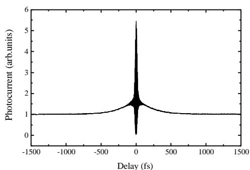
**Fig. 3.** Signal trace obtained with a PMT R2557. It has tails with a decay time of 270 fs, which can be regarded as the lifetime of the intermediate state of the two-photon-induced process.
