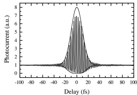
**Fig. 2.** Interferometric autocorrelation trace of 15-fs, 800-nm pulses from a Ti:sapphire laser obtained with a 1P28 photomultiplier tube at input power as low as 410  $\mu\text{W}$ . Simulated envelopes of the autocorrelation trace of 15-fs Gaussian pulses are also shown.
