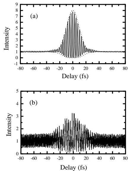
**Fig. 1.** Interferometric autocorrelation trace of 15-fs, 800-nm pulses from a Ti:sapphire laser obtained by measurement of two-photon-induced photocurrent in a GaAsP photodiode at input power of (a) 70 mW and (b) 500  $\mu\text{W}$ .
