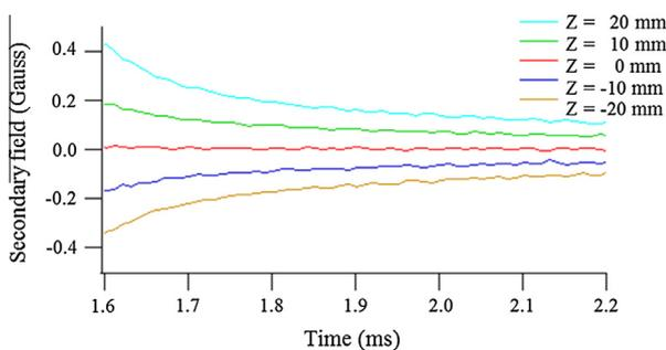
Fig. 15. Eddy current fields as a result of eddy currents induced in components of the MRI system other than the local RF shielding box.
