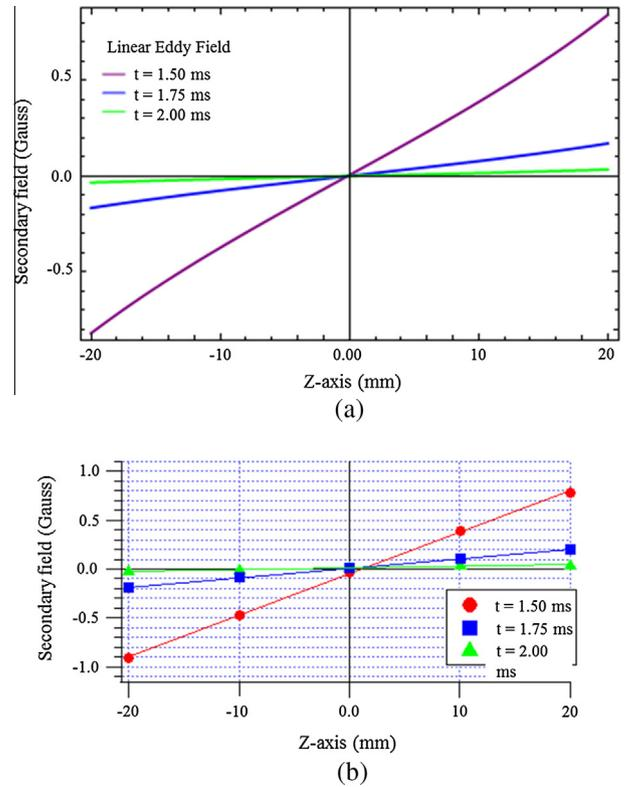
**Fig. 9.** Linear eddy field responses for three different time instants calculated after the end of the applied gradient current. Good agreement was found between (a) simulation and (b) experimental results.
