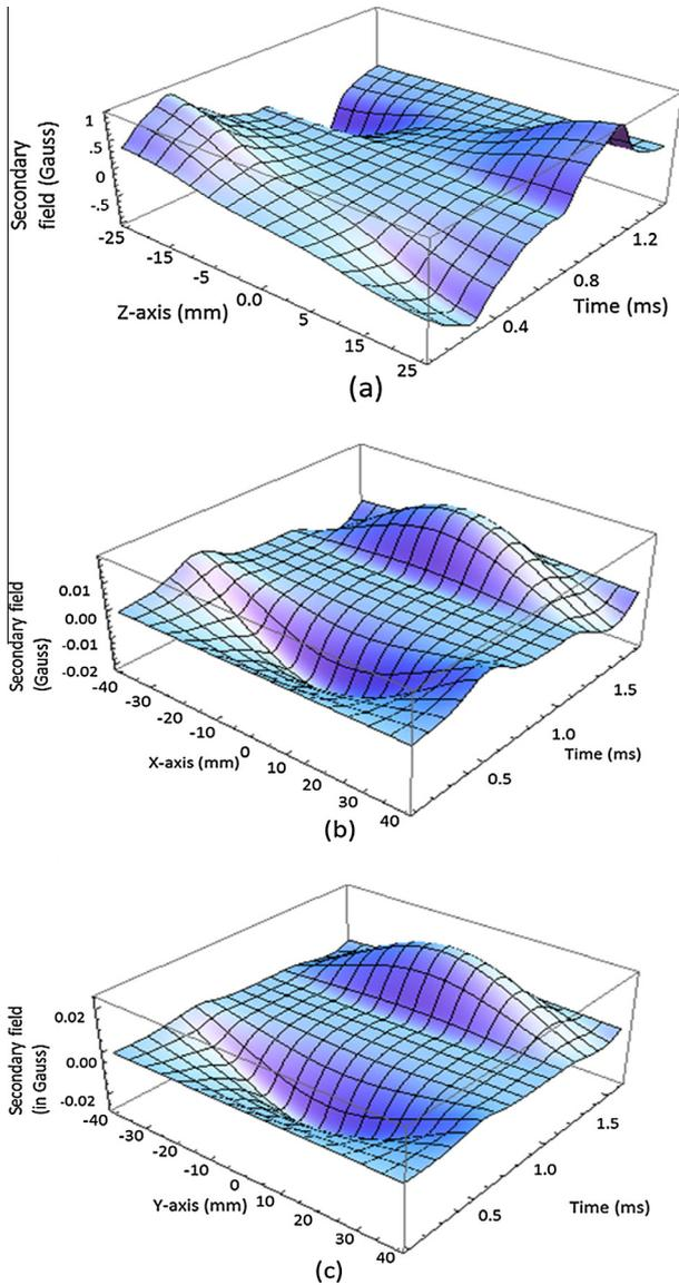
Fig. 10. Secondary transient magnetic fields along the (a) Z-axis, (b) X-axis, and (c) Y-axis in the ROI as a result of Z-gradient-induced eddy currents in the RF shielding box.
