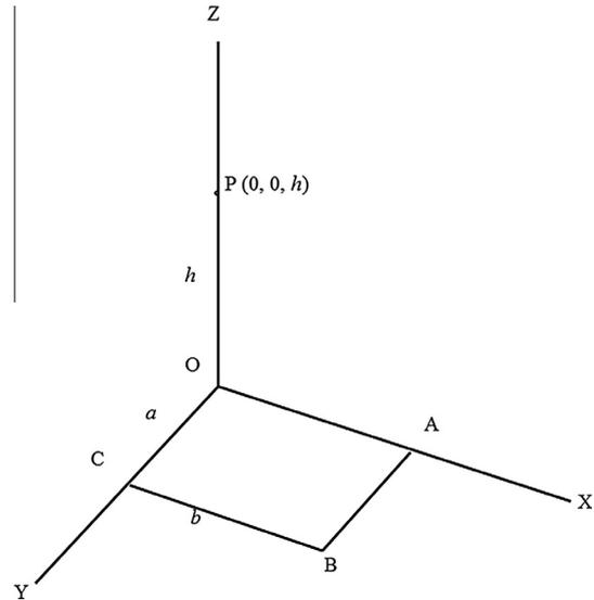
Fig. C1. Geometry for the calculation of solid angle subtended by a rectangular section ABCO at a distance  $h$  on the Z-axis.
