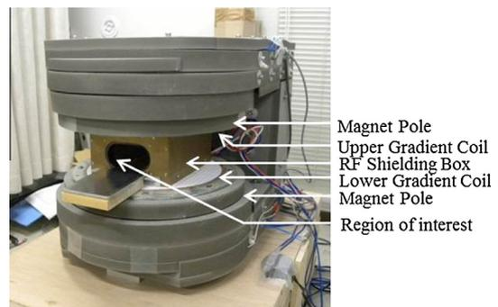
Fig. 1. Open compact 0.3 T magnetic resonance imaging (MRI) system for skeletal age assessment in children.
