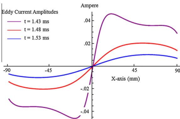
Fig. 11. Eddy current distribution along the X-axis induced by X-gradient coil. In accordance with the field response of the X-gradient coil, the distributed eddy currents were found to be nearly zero at the center of the brass plate and increasing or decreasing values on opposite sides from the center.
