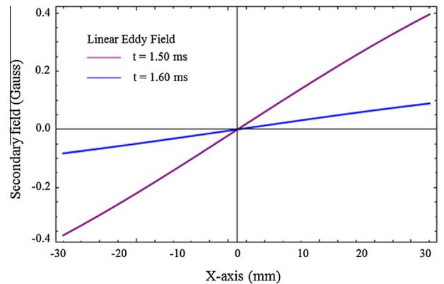
Fig. 14. Linear secondary magnetic field induced by X-gradient coil.
