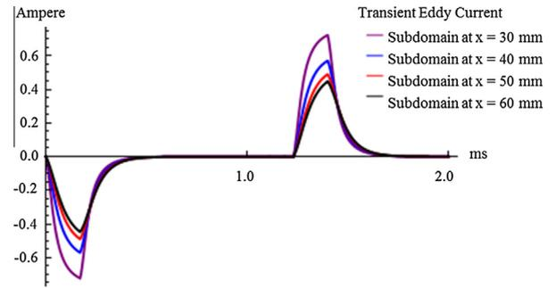
Fig. 12. Eddy current transient response induced by X-gradient coil. Here responses are given for few subdomains located at different position on the X-axis.
