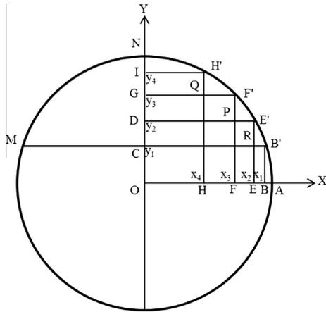
**Fig. C3.** Rectangular segmentation approach in the calculation of solid angle subtended by the X- or Y-gradient coil. Here half of the area of a coil is divided into several rectangular sections. The total solid angle would be twice of the solid angle subtended by this portion in first quadrant.
