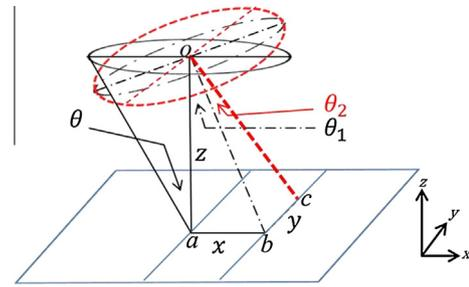
Fig. B2. Geometric representation of a solid angle calculation in the X–Y plane. The dotted schematics represent the inclinations of the coil to account for the projection of the solid angle considering any point in the X–Y plane.  $\theta_1$  and  $\theta_2$  are the projection angles for any point along the X- and Y-axis, respectively, and  $ab$  and  $bc$  are the distances from the center along the X- and Y-axis, respectively.
