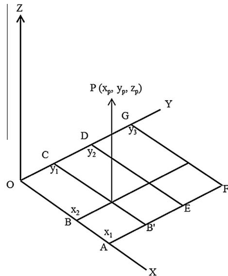
Fig. C2. Geometry for the calculation of solid angle subtended by an arbitrary rectangle at any field point  $P(x_p, y_p, z_p)$ .
