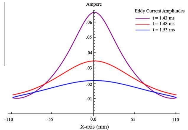
Fig. 5. Eddy current amplitudes along (a) the X-axis in the upper plate of the RF shielding box. The plate was subdivided into sublayers along the thickness (along the Z-axis). Here, results are given for the outermost layer. A symmetric current distribution from the center of the plate is seen in the diagram.
