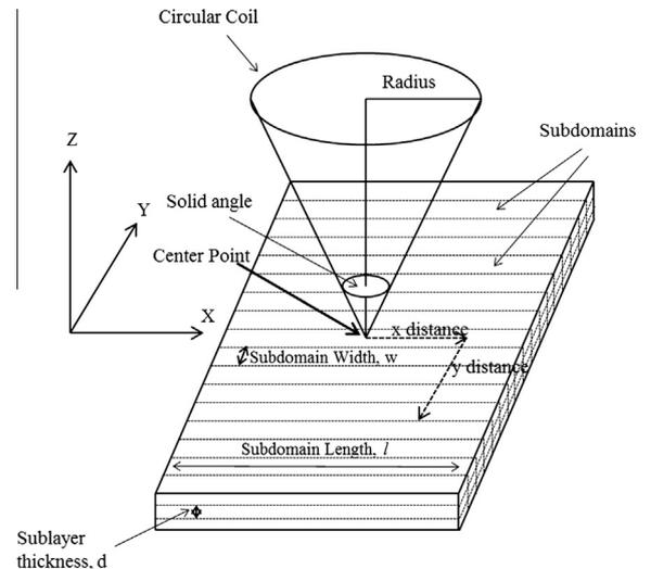
Fig. 3. A schematic representation of the solid angle approach implemented in the coupled circuit numerical method is shown for a circular turn of coil. Imaginary slices are considered as inductively coupled subdomains of minimal thickness.
