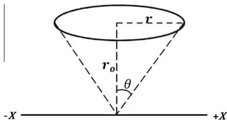
Fig. B1. Geometric representation of the solid angle of a circular coil. Here,  $\theta$  is the apex angle of the solid angle subtended at a distance  $r_0$  by a circular coil of radius  $r$ .
