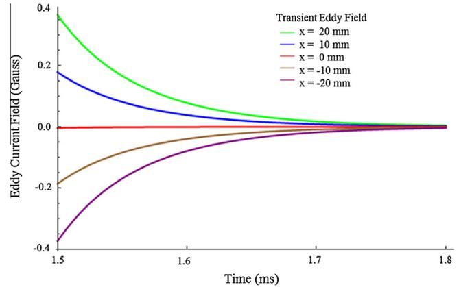
Fig. 13. The X-gradient coil generated eddy current field is illustrated here for few points along the X-axis. X-gradient generated eddy field decays faster than the Z-gradient induced secondary magnetic field.
