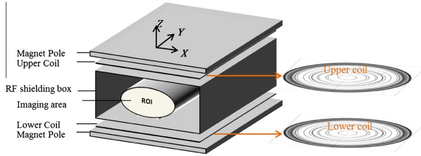
**Fig. 2.** Schematic representation of the open compact MRI system. The planar gradient coil consisted of an upper and a lower coil, shown separately on the right side of the diagram. The local RF shielding box is positioned in between these coils. Eddy currents are expected to be created in the brass plates of the boundary of the RF box, and the secondary magnetic fields created by these eddy currents have a major effect on the region of interest (ROI).
