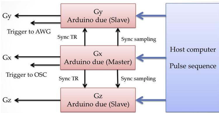
**Fig. 3** Block diagram of the pulse programmer using three microcontroller boards. The master microcontroller generates the exact timing for the repetition time (TR) and for pulse programmer events that are synchronized with the slave microcontrollers using digital input/output pins
