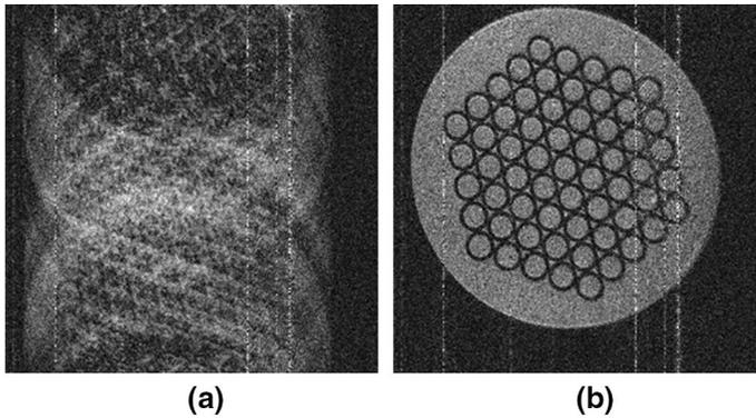
**Fig. 7** 2D MR images acquired using type A console **a** without and **b** with phase correction. TR = 400 ms, TE = 11.9 ms, slice thickness = 5 mm, FOV = 35 mm × 35 mm, matrix size = 256 × 256. The vertical line noise is external noise
