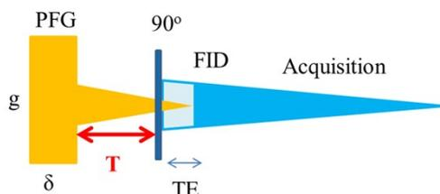
Fig. S1. The pulse sequence to estimate the eddy current effects. The interval time  $T$  between PFG and  $90^\circ$  pulse was set variable.
