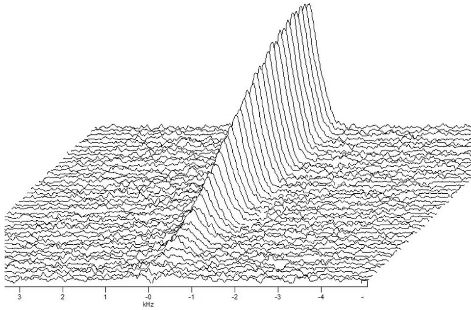
Fig. S6. Echo attenuation spectra of the LAGP at 38 °C in real mode measured with  $\Delta = 15$  ms,  $g = 14.3 \text{ Tm}^{-1}$ ,  $\delta = 0.1$  to 4 ms (40 points), and  $\tau = 4.5$  ms.
