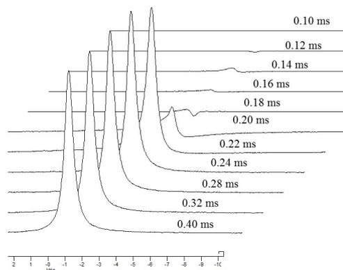
Fig. S2.  $^7\text{Li}$  spectral patterns for  $\text{TE} = 0.1 \text{ ms}$ ,  $\delta = 2 \text{ ms}$ ,  $g = 10.0 \text{ Tm}^{-1}$ , and  $T = 0.10$  to  $0.40 \text{ ms}$ .
