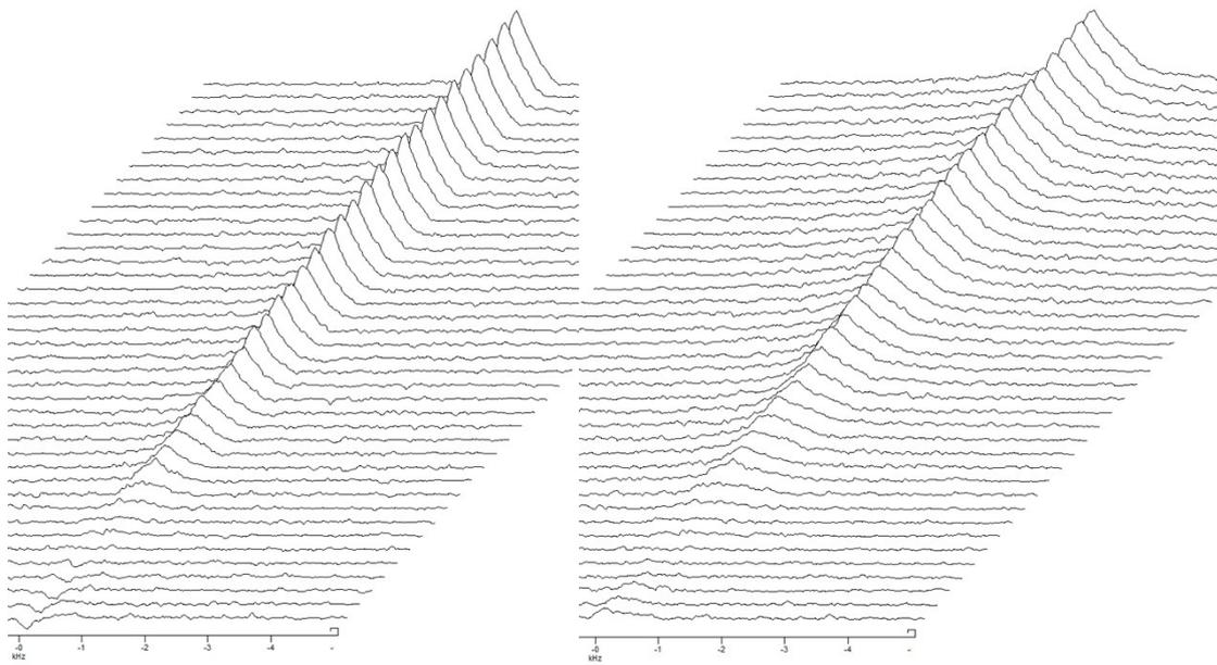
Fig. S7. Echo attenuation spectra of the LAGP at 38 °C measured with  $\Delta = 15$  ms,  $g = 10.0 \text{ Tm}^{-1}$ ,  $\delta = 0.1$  to 4 ms (40 points), and  $\tau = 4.5$  ms. **Left:** real mode and **right:** magnitude mode. The echo signals changed their phases near the diffraction and the peak heights of the negative signals disappear in logarithmic plots. The signals with the magnitude mode were used for the echo attenuation plots in Figs. 4, 8, and S8.
