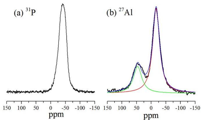
Fig. S4. (a)  $^{31}\text{P}$  and (b)  $^{27}\text{Al}$  spectra of LAGP at 30 °C. The  $^{31}\text{P}$  and  $^{27}\text{Al}$  shifts were referred to  $\text{H}_2\text{PO}_4$  and  $\text{AlCl}_3$  in aqueous solutions, respectively.
