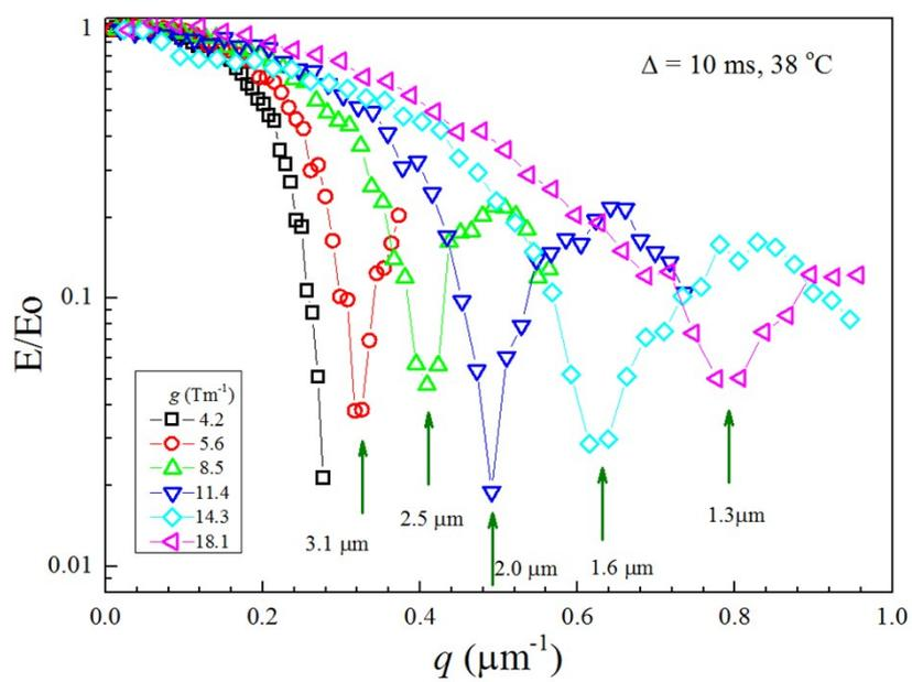
Fig. S8. The echo attenuation plots on  $\Delta = 10 \text{ ms}$  at  $38 \text{ }^\circ\text{C}$  measured with a fixed  $g$ -value and varying  $\delta = 0.1$  to  $4.0 \text{ ms}$  (40 points) for  $g = 18.1$  (left-triangle),  $14.3$  (diamond),  $11.4$  (down-triangle),  $8.5$  (up-triangle),  $5.6$  (circle) and  $4.2 \text{ Tm}^{-1}$  (square). The measurements were also performed for  $g = 12.9$ ,  $10.0$ , and  $7.1 \text{ Tm}^{-1}$ .
