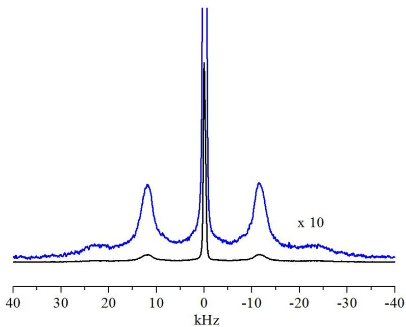
Fig. S5.  $^7\text{Li}$  NMR spectrum in the wide range for the LAGP at 30 °C.
