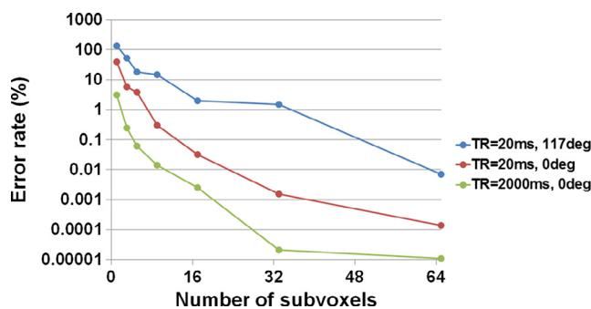
**Fig. 10.** Error rate plotted against the number of subvoxels for the RF spoiled gradient echo sequence with (a) TR = 20 ms and  $\Phi = 117^\circ$  (conventional SPGR) shown in blue, (b) TR = 20 ms and  $\Phi = 0^\circ$  (conventional gradient-echo sequence) shown in brown, and (c) TR = 2000 ms and  $\Phi = 0^\circ$  shown in light green. (For interpretation of the references to colour in this figure legend, the reader is referred to the web version of this article.)
