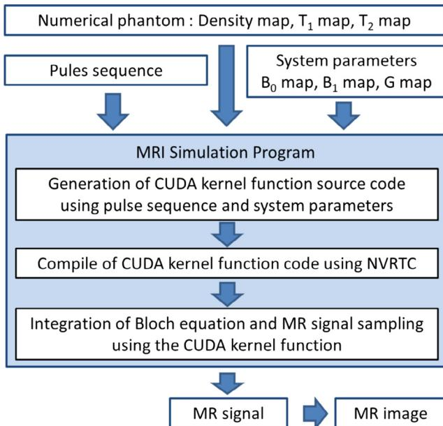
**Fig. 1.** Structure of BlochSolver. The input data are the numerical phantom, the pulse sequence, and the system parameters. CUDA kernel function code, generated automatically using the pulse sequence and the system parameters, is compiled to execution code for the GPU using NVRTC (NVIDIA runtime compilation library). The Bloch equation is integrated to calculate the NMR signal for the MR image.
