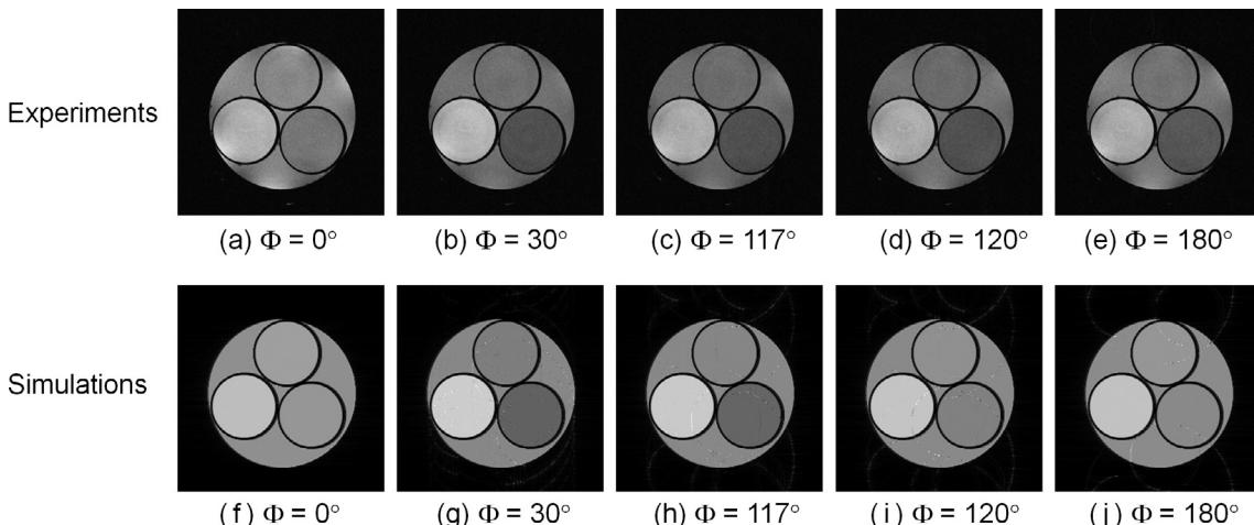
**Fig. 11.** Cross-sectional images selected from 3D image datasets acquired with the SPGR sequences (TR/TE = 20 ms/6 ms, FA = 30°, image matrix =  $256 \times 256 \times 32$ , FOV =  $[64 \text{ mm}]^3$ ).  $\Phi$  was the phase increment angle described in the text. (a)–(e) acquired by experiment at 1.5 T. (f)–(j) calculated with BlochSolver (without diffusion effects). The number of subvoxels was 65. The execution time for one SPGR image was about 156 s.
