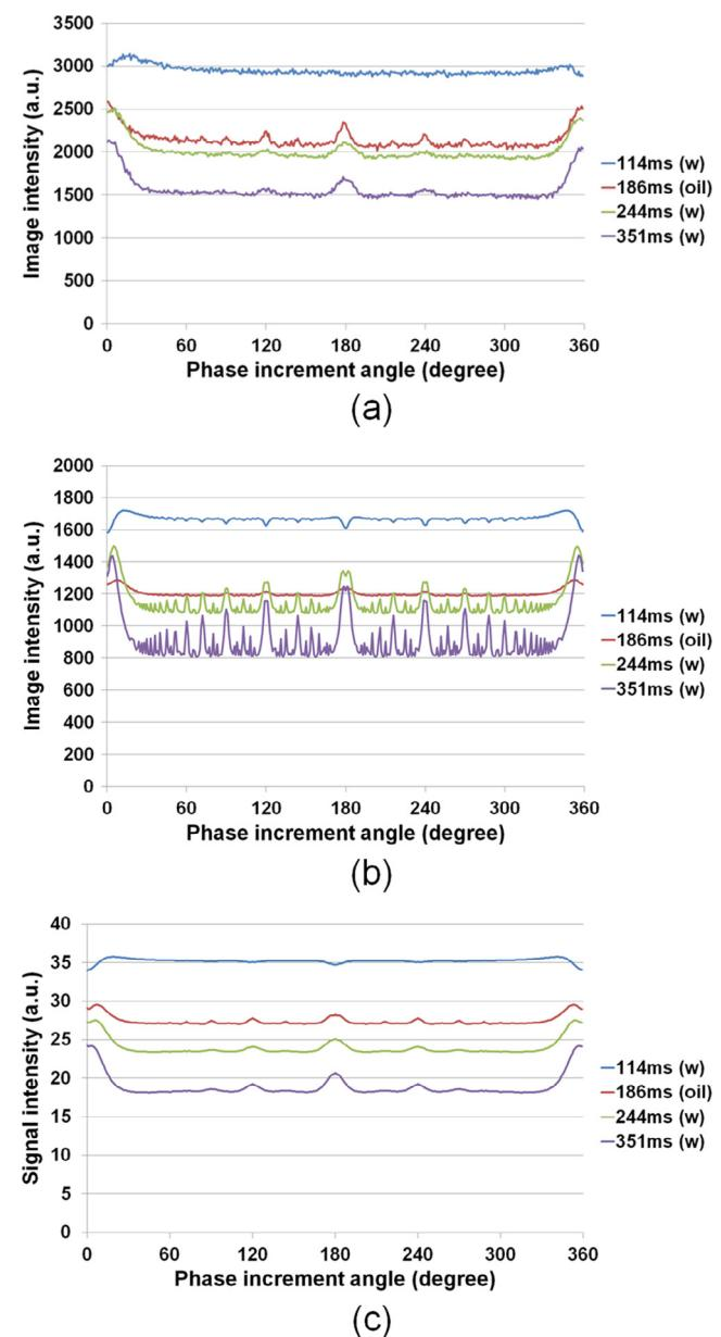
**Fig. 12.** Phase increment angle dependence of the image intensity in the relaxation phantom. (a) Experiments. (b) Simulations without molecular diffusion effects. (c) One voxel simulation with a molecular diffusion effect. The numbers written in the legends of the graphs are  $T_1$  values.
