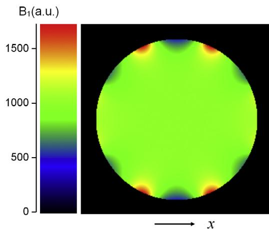
**Fig. 6.** Theoretically calculated  $B_1$  map of the linear-drive birdcage coil. The direction of the RF magnetic field is parallel to the x direction. The field of view is  $(64\text{ mm})^2$ . Diameter of the birdcage coils is 64 mm. The diameter of the circle shown above is 54 mm.
